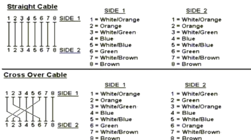
Figure A-1: Straight-Through and Crossover Cable
